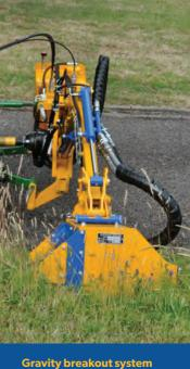
For protecting drive and machine during operation.
