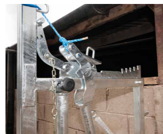
RATCHET LOCKING POINTS FOR THE YOKE
