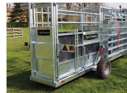
9. FOLD AWAY BRAKE LIGHTS Included as standard so can be used on the road straight away
