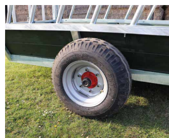
10.0 75 X 15.3 6-STUD WHEELS ON 60MM STUB AXLES
