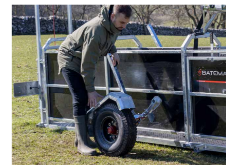
10. REMOVABLE AXEL To give full access to the race
