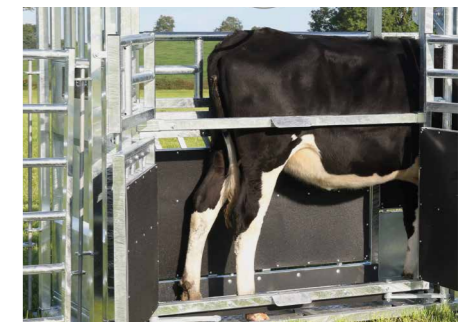
8. SIDE DOORS Full access spring loaded side doors
