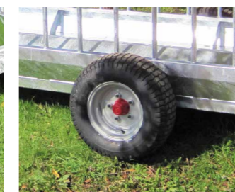
23 X 10.5 -12 5-STUD WHEELS ON 50MM STUB AXLES
