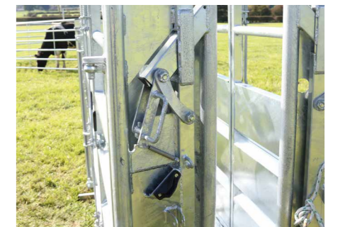
8. YOKE WIDTH ADJUSTMENT Six easy to change settings
