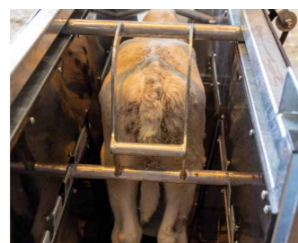
BACK UP BAR INCLUDED WITH 4 FIXING POINTS FOR DIFFERENT SIZE ANIMALS
