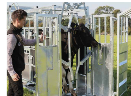
6. YOKE LOCKED IN PLACE Scissor style manual yoke
