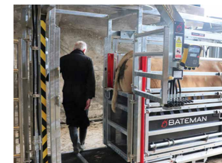
10. ACCESS KIOSK Split gates can close behind the animal to provide safe access
