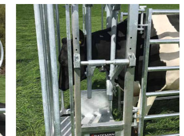
SAFETY CAGE AROUND THE FRONT OF THE YOKE
