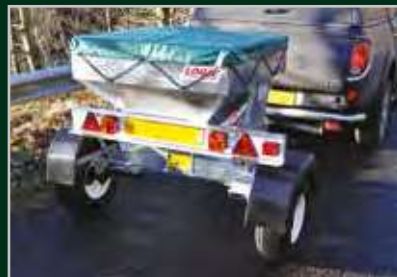
Model LMF610R with suspension axles, road wheels, lighting board and optional LMF101 tonneau cover.
