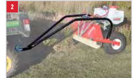
The robust 'swan neck' drawbar reduces drag in dense foliage. It can be easily moved to provide an offset facility and houses the large, in-line filter.
