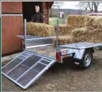
XRT740 with 195x60-R14 wheels and tyres, showing optional XT202 mesh hinged sides, XT202-10A wire kit and XT106 mesh ramp tailgate. Ideal for bulky loads like these straw bales.
