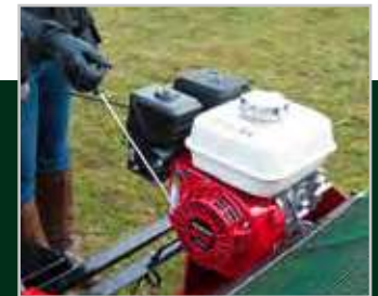
The MSP120 is powered by a Honda 5.5hp engine, with its legendary reliability and easy pull start system. This power unit gives the sweeper complete independence so that it can be towed by any suitable vehicle, depending on the location and conditions.
