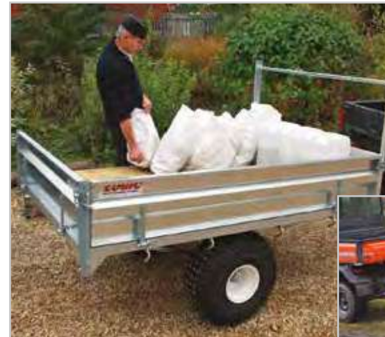
STT400 trailer 1500 x 1000 x 380mm with STT103 tailgate.
