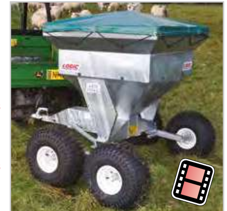
LMF570TA tandem axle model (above) with optional LMF108 hopper extension and LMF109 tonneau cover. This wheel layout improves the smoothness of travel and stability over rough ground. Seen here with optional extension sides to increase capacity to 625 litres.
