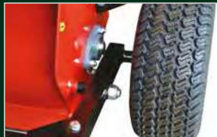
Wide rear castor wheels ensure specialist grassed surfaces are not damaged.
