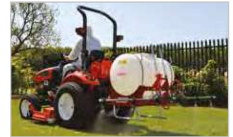
Perfect for small tractors with 'Cat 1' linkages like this compact tractor mower unit. The skid unit sets the sprayer at a good height for dismantling and storage.
