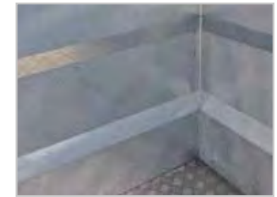
All-welded monocoque construction with aluminium 'tread plate' floor for safety, lighter weight benefits and easy cleaning for bio-security purposes.
