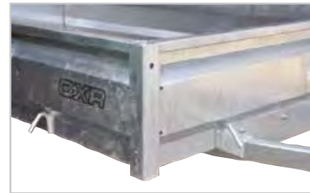
Strong monocoque construction with rope hooks and high quality galvanising for long life protection.
