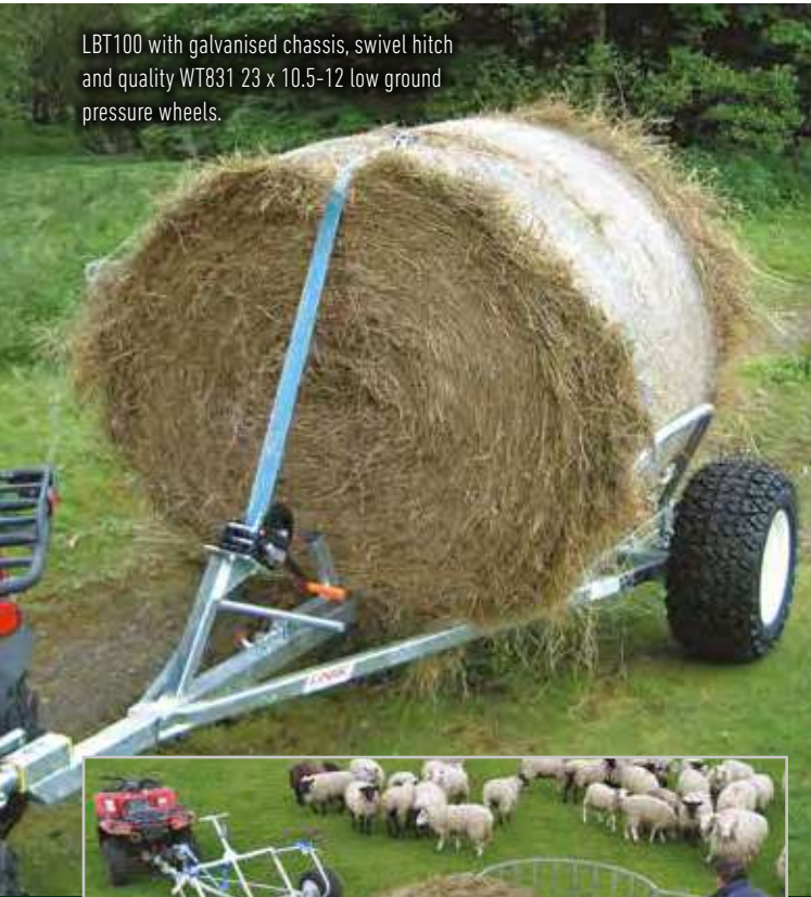
1 Back up to bale, secure strap
