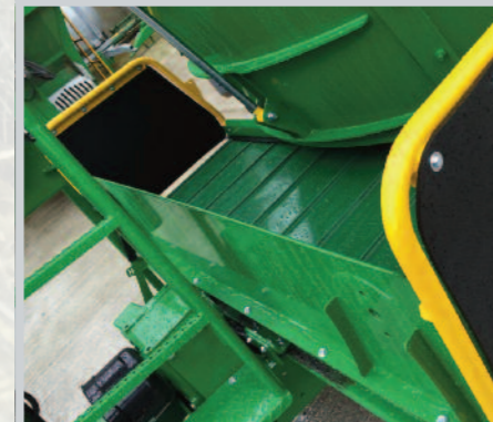
Front PVC conveyor
