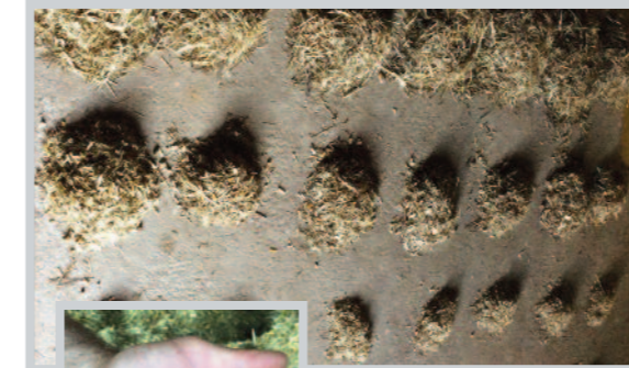
Picture above shows a series of tests made over several hours to show the composition of the feed does not change with our feeder.
