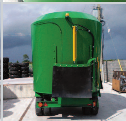
Additional discharge door
